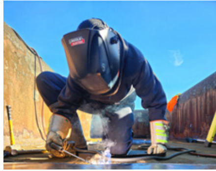
Sabian Darke welding patches inside a gondola in The Rip.
