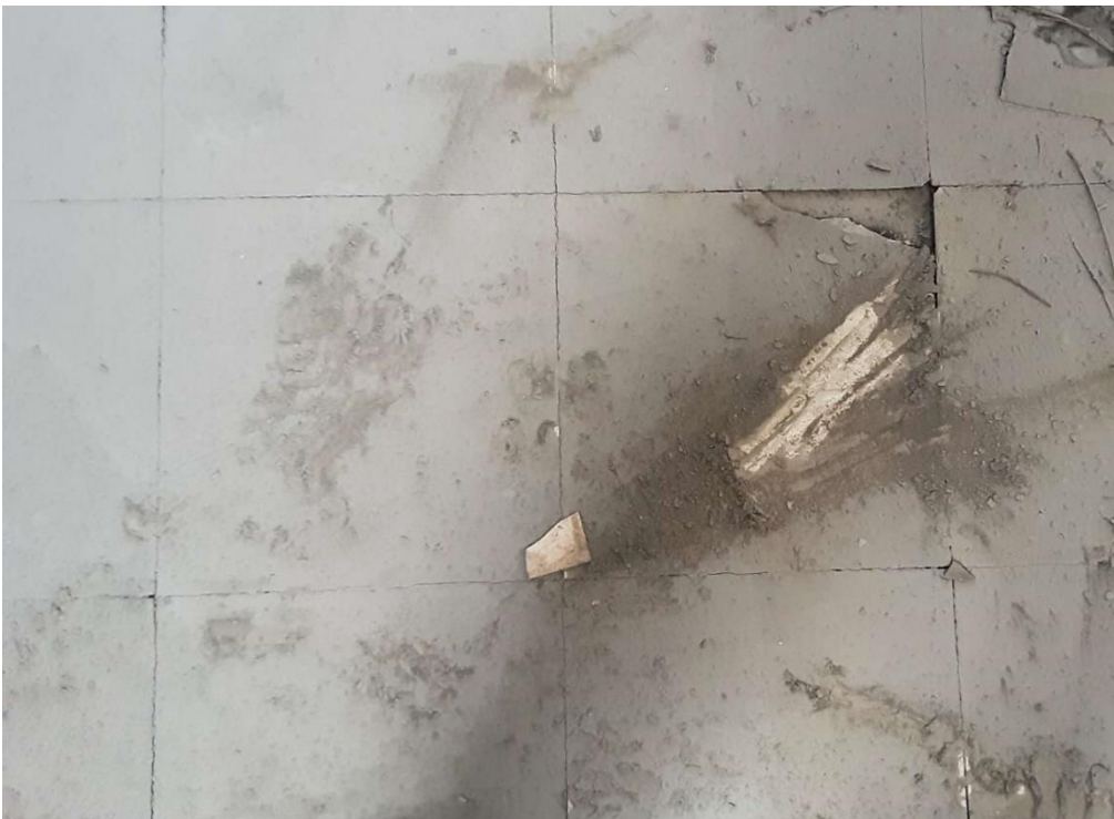
S0004C (Confirmed Asbestos), 12" x 12" White, Floor, Vinyl Floor Tile, Storage (Location #: 4)
