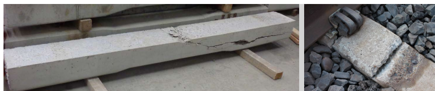
Figure SUB-PART D – 6 – Broken Through Concrete Tie (left) and Transversely Broken Concrete Tie Between Rails (right)
