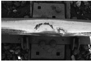
Figure SUB-PART D – 38 – Crushed Head (left) and Straight Edge Placement (right)
