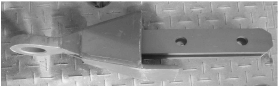
Figure SUB-PART D – 59 – Rail Shoe (used to pull rail through the threader box)
