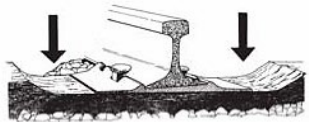
Tie Adzed to a Depth of 2" or Greater
